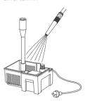
The tank and pump must be free of dirt.
